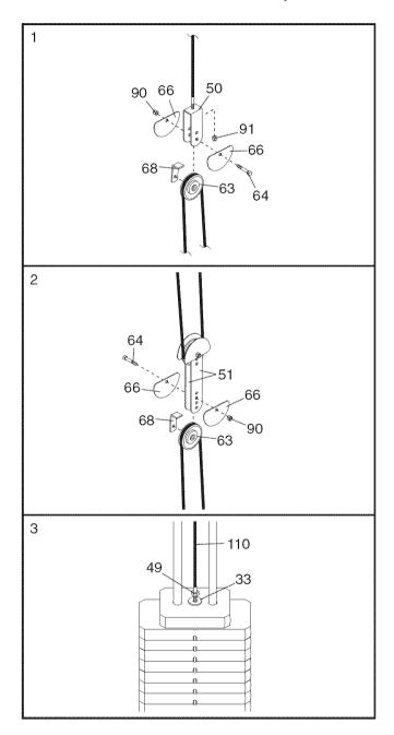
Do not overtighten the cables. If the cables are overtightened, the top weight will be lifted off the weight stack. If a cable tends to slip off the pulleys often, it may have become twisted. Remove the cable and re-install it. If the cables need to be replaced, see the part ordering information on the back cover of this manual.
